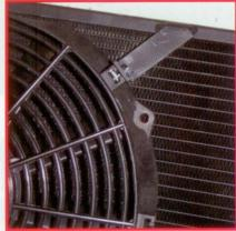
vulnerable position where they might get pebble-dashed by stones as they aren't as robust as copper and brass (brass tank and tubes with copper fins). Aluminium radiator cores are brazed together and are more efficient than copper and brass cores held together with lead solder (which makes them less efficient).
